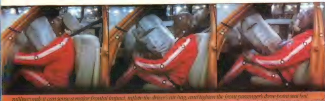
milliseconds: it can sense a major frontal impact, inflate the driver's air bag, and tighten the front passenger's three-point seat belt.
